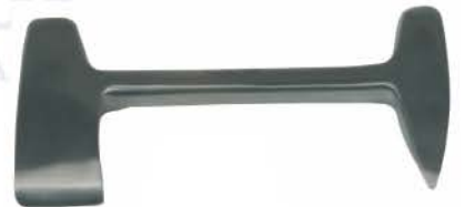
BT1-096 clinch cutter. 6" double ended tool for opening the clinches to reduce hoof wall damage during shoe removal. Beveled on inside edge for closer cutting. Stainless. Other end is
